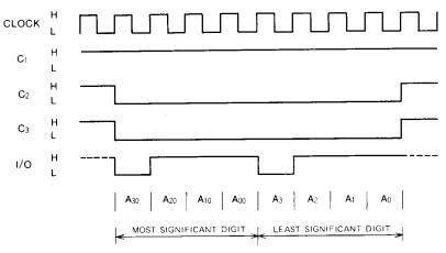
Note 2: The addresses from  $A_{00}$  to  $A_{33}$  are designated by two one-of-four coded digits. The above figure shows designation of address  $A_{33}$  (decimal address 15).
