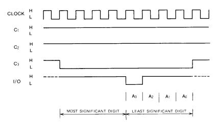
Note 3. In the AD accept address mode, the higher four are set high, and the lower four digits are designated by one of the four coded digits. This address mode allows designation of addresses from  $A_{\rm b}$  to  $A_{\rm 3}$ . Each address has a 16 bits. The above figure shows designation of address  $A_{\rm 3}$ .
