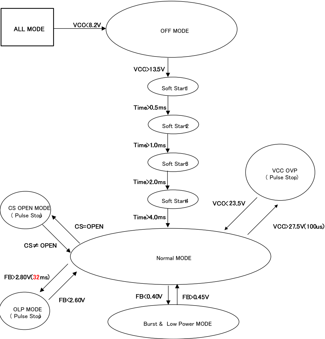
Figure 18. The sequence diagram (BM1PXX1 Series)
